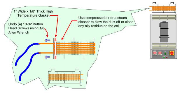
To clean the cooling coil, use compressed air or a steam cleaner to blow the dust off or clean any oily residue on the coil.
